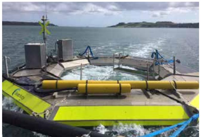
Seatricity's Oceanus 2 device being installed at WaveHub (courtesy of RegenSW)
