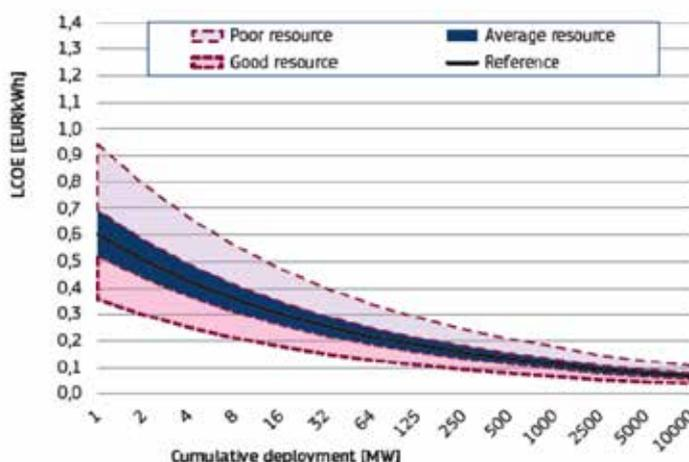
LCOE predictions for tidal arrays. Source: JRC based on ERTI 2014
